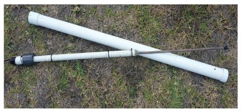
I won't go into a step by step build of how the wbole thing is put together, but I feel the photo of the antenna without the weather covers is self explanatory. Note that the pvc sleeve extends through the 50-20 mm grey pvc coupling (the ridge inside the coupling needs removal to allow the conduit to pass through - or 2 sections could be cemented into place).
